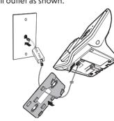
Alian the holes on the bracket with the standard wall plate and slide the bracket down until it clicks securely in place.
