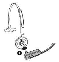
Rotate the headset to vertical direction until it clicks into place.
