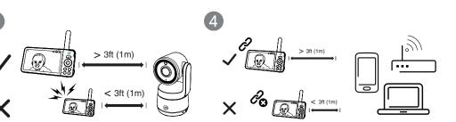
To avoid interference from other electronic devices, place your baby monitor at least 3 feet (1 meter) away from devices such as wireless routers, microwaves, cell phones and computers.
