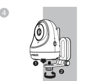
Place the baby unit on the wall mount bracket. Tighten the screw into the threaded socket at the bottom to secure the baby unit.
