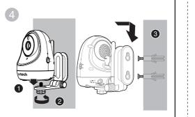
Place the baby unit on the wall mount bracket. Tighten the screw into the threaded socket at the bottom to secure the baby unit. Align the holes on the wall mount bracket with the screws on the wall, and slide the wall mount bracket down until it locks into place.
