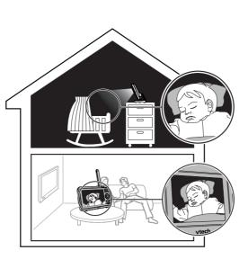
The baby unit has infrared LEDs that allow you to see your baby clearly at night or in a dark room. When the baby unit being viewed detects low light levels, the infrared LEDs are switched on automatically. The images from the baby unit are in black and white, and appears on the screen.
