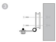
Alian the wall mount bracket and screws with the holes in the wall as shown. Tighten the screw in the middle hole first, so that the wall mount bracket position is fixed. You can tighten the other screw in the top hole.
