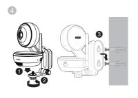
Place the baby unit on the wall mount bracket. Tighten the screw into the threaded socket at the bottom to secure the baby unit. Alian the holes on the wall mount bracket with the screws on the wall, and slide the wall mount bracket down until it locks into place
