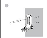
Place the wall mount bracket on a wall and then use a pencil to mark the top and the bottom holes as shown. Remove the wall mount bracket and drill two holes in the wall (7/32 inch drill bit).
