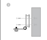
Align the wall mount bracket and screws with the holes in the wall as shown. Tighten the screw in the middle hole first, so that the wall mount bracket position is fixed. You can tighten the other screw in the
