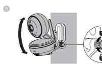
The default angle of the wall mount bracket is 90 degrees. You can maximize your baby unit's viewing angles by tilting the wall mount bracket.
