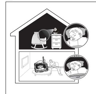
The baby unit has infrared LEDs that allow you to see your baby at night or in a dark room. When the baby unit detects low light levels, the infrared LEDs turn on automatically. The images from the baby unit are in black and white, and  $\sqrt[3]{}$  appears
