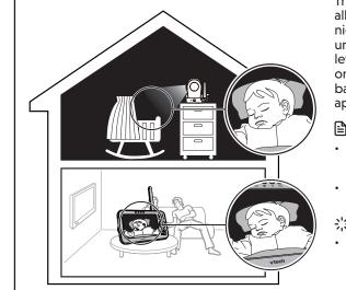
The baby unit has infrared LEDs that allow you to see your baby clearly at night or in a dark room. When the baby unit being viewed detects low light levels, the infrared LEDs are switched on automatically. The images from the baby unit are in black and white, and  $extcolor{}$ appears on the screen.
