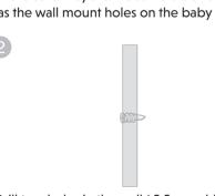
Drill two holes in the wall (5.5 mm drill bit). If you drill the holes into a stud, go to step 3.
