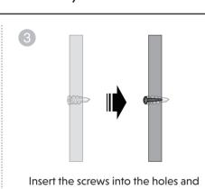
tighten the screws until only 6.5 mm of the screws are exposed.
