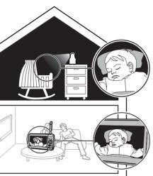
The baby unit has infrared LEDs that allow you to see your baby clearly at night or in a dark room. When the baby unit being viewed detects low light levels, the infrared LEDs are switched on automatically. The images from the baby unit are in black and white, and 🥨 appears on the parent unit screen. NOTES
