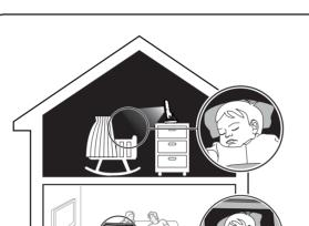
The baby unit has infrared LEDs that allow you to see your baby clearly at night or in a dark room. When the baby unit being viewed detects low light levels, the infrared LEDs are switched on automatically. The images from the baby unit are in black and white, and 2 ppears on the screen.
