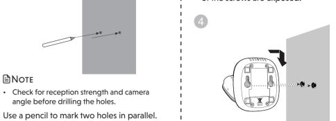
Align the wall mount holes on the baby unit with the screws on the wall. Slide the baby unit down until it locks into place.
