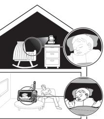
The baby unit has infrared LEDs that allow you to see your baby clearly at night or in a dark room. When the baby unit being viewed detects low light levels, the infrared LEDs are switched on automatically. The images from the baby unit are in black and white, and 🥝 appears on the screen. It is normal to see a short white glare on
