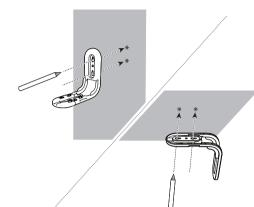
2. Remove the wall mount bracket and then drill two holes in the wall or on the ceiling (7/32" drill bit).
