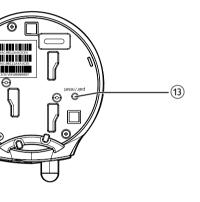
1. Connect the power adapter to the camera unit and a power supply.
